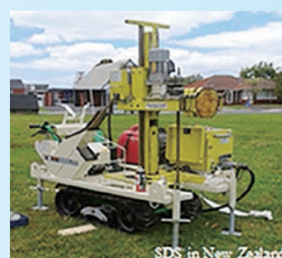
Screw Drive Sounding
