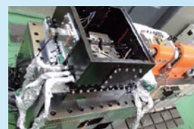
Friction force measurement and seizure evaluation unit system for plain bearings
